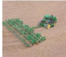
A **plow** has long blades that loosen and turn over the soil and kill weeds.
