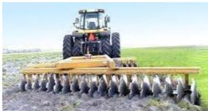
A **harrow** has discs that help to smooth the soil by breaking up large clumps, making it easier for new plants to grow.
