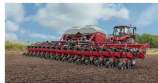
A **seed planter** is used to plant seeds quickly over large areas. The seed planter sows and buries seeds in equally spaced rows.
