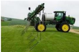
A **liquid fertilizer spreader** adds fertilizer to the soil to increase the nutrients needed for crops to grow.
